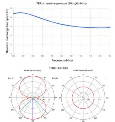
Trace-ID's UHF RFID tag TER17 with IMPINJ M700 Chip series was developed to improve performance of its predecessor and suits RFID solutions for Returnable Transport Units, supply chain, logistics, and inventories. It's also appropriate for retail itemlevel deployments like apparel traceability.
